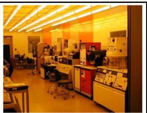
The NFC clean room contains a wide variety of equipment for building micro and nano scale devices.
