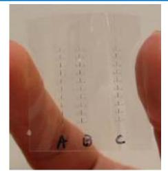
Printed transistors on plastic using high capacitance, nanostructured gate dielectrics by Professors C. Dan Frisbie, (CEMS), and Tim Lodge, (Chem). Printed transistors show lowvoltage operation and high on-current.
