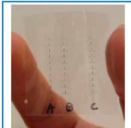
Printed transistors on plastic using high capacitance, nanostructured gate dielectrics by Professors C. Dan Frisbie, (CEMS), and Tim Lodge, (Chem). Printed transistors show low-voltage operation and high on-current.
