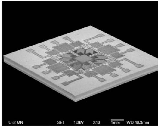
Professor Rajesh Rajamani (ME) designed and built a novel micro electro mechanical system (MEMS) angle sensor that measures inertial angle directly instead of angular rate. It can be used for a variety of positioning and navigation applications.
